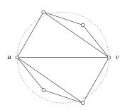
Figure 101: The edge uv is locally Delaunay but does not belong to the Delaunay triangulation.
