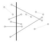
Figure 96: Five of the line segments intersect the sweep-line at its current position and two of them cross.
