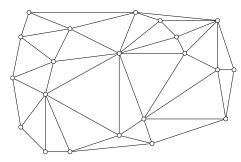
Figure 98: Delaunay triangulation of the same twenty-one points triangulated in Figure 97.
