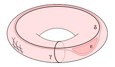
Figure 88: The 1-cycles  $\gamma$  and  $\delta$  are not 1-boundaries. Adding the 1-boundary  $\varepsilon$  to  $\delta$  gives a 1-cycle homologous to  $\delta$ .
