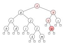
Figure 12: The shaded nodes indicate the path from the root we traverse when we insert w into the sorted tree.
