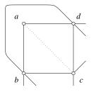
Figure 74: Drawing the edge from a to c decomposes the quadrangle into two triangles. Note that we cannot draw the edge from b to d since it already exists outside the quadrangle.
