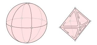
Figure 81: A triangulation of the sphere. The eight triangles are glued to form the boundary of an octahedron which is homeomorphic to the sphere.
