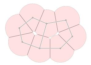
Figure 105: The Voronoi decomposition of a union of eight disks in the plane and superimposed dual alpha complex.
