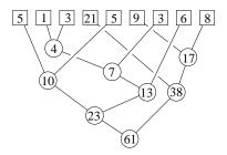
Figure 8: The numbers in the external nodes (squares) are the weights of the corresponding letters, and the ones in the internal nodes (circles) are the weights of these nodes. The Huffman tree is full by construction.
