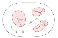
Figure 65: The vertices inside and outside the shaded regions form a cut that respects the collection of solid edges. The dotted edges cross the cut.
