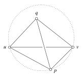
Figure 102: The edge uv is non-lD and can be flipped to the edge pq, which is lD.
